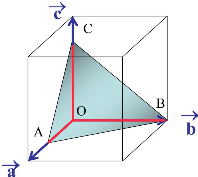
$$\left. \begin{array}{l} OA = 1/2 a \\ OB = 1 b \\ OC = 3/4 c \end{array} \right\} \Rightarrow \begin{array}{l} h \propto 2 \\ k \propto 1 \\ l \propto 4/3 \end{array}$$
