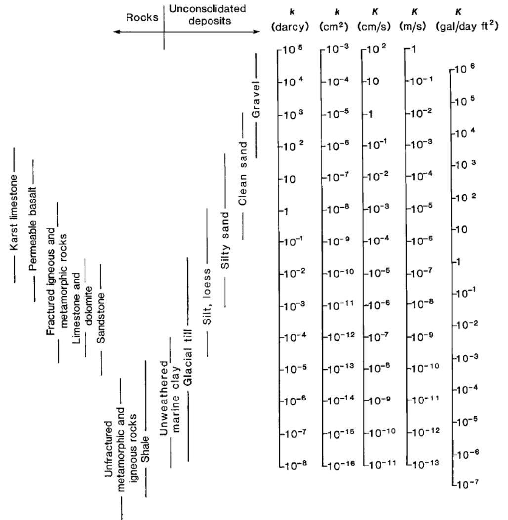
Figure 5.8 Range of values of hydraulic conductivity and permeability. Reproduced from Freeze, R.A. and J.A. Cherry, Groundwater, p. 604 © 1979 Prentice Hall.
