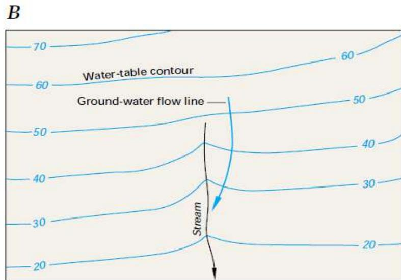
*Figure 8. Gaining streams receive water from the ground-water system (A). This can be determined from water-table contour maps because the contour lines point in the upstream direction where they cross the stream (B).*
