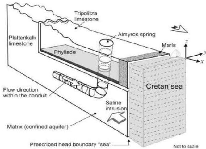
**Figure 3.** Schematic 3-D view of the coastal karstic aquifer of the Almyros of Heraklio spring.
