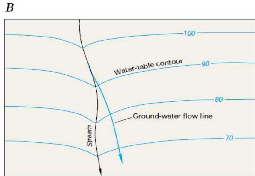
*Figure 9. Losing streams lose water to the ground-water system (A). This can be determined from water-table contour maps because the contour lines point in the downstream direction where they cross the stream (B).*
