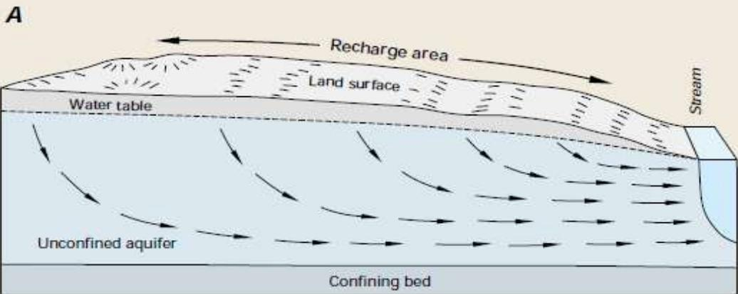
Figure C-1. In a schematic hydrologic setting where ground water discharges to a stream under natural conditions (A), placement of a well pumping at a rate ( $Q_1$ ) near the stream will intercept part of the ground water that would have discharged to the stream (B). If the well is pumped at an even greater rate ( $Q_2$ ), it can intercept additional water that would have discharged to the stream in the vicinity of the well and can draw water from the stream to the well (C).
