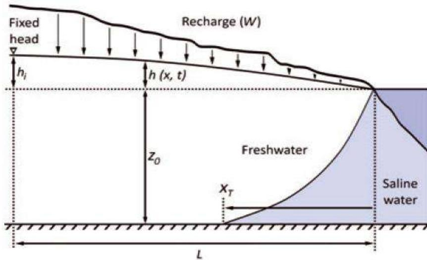
Figure 1. Conceptual model of a coastal aquifer controlled by an inland fixed-head ( $h_i$ ).
