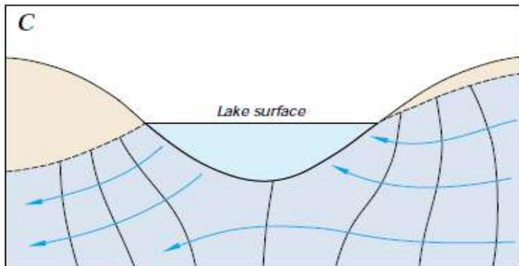
*Figure 16. Lakes can receive ground-water inflow (A), lose water as seepage to ground water (B), or both*
