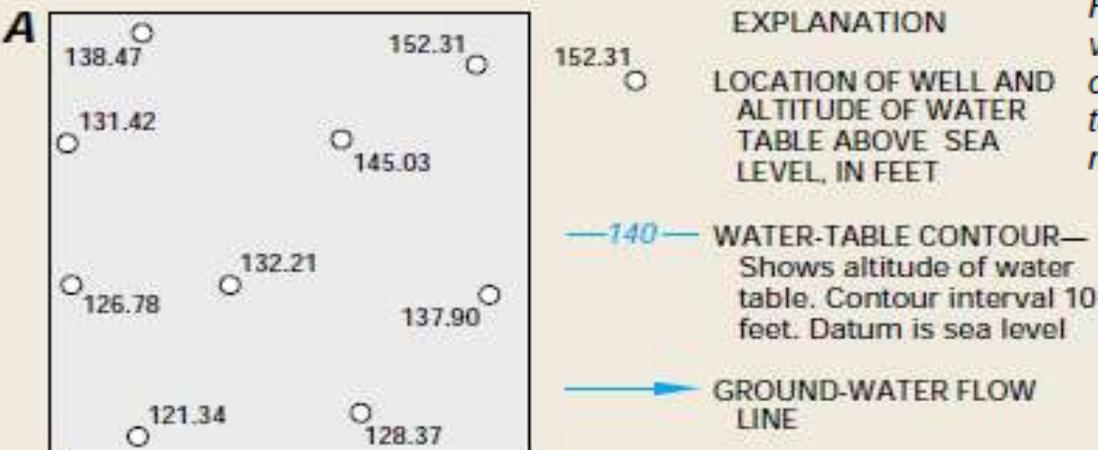
Figure A-2. Using known altitudes of the water table at individual wells (A), contour maps of the water-table surface can be drawn (B), and directions of ground-water flow along the water table can be determined (C) because flow usually is approximately perpendicular to the contours.
