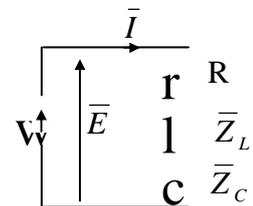
$$\varphi = \text{Arg}(\bar{I}) = \text{Arg}(\bar{E}) - \text{Arg}(\bar{Z}) = 0 - \text{Arctg} \left( \frac{L\omega - \frac{1}{C\omega}}{R} \right) = \text{Arctg} \left( \frac{1 - LC\omega^2}{RC\omega} \right)$$
