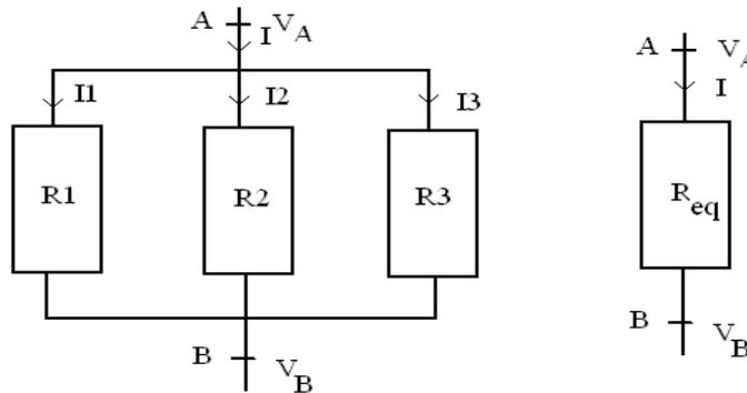
$$V_A - V_B = R_1 I_1 = R_2 I_2 = R_3 I_3 = R_{eq} I \quad \text{or} \quad I = I_1 + I_2 + I_3$$
